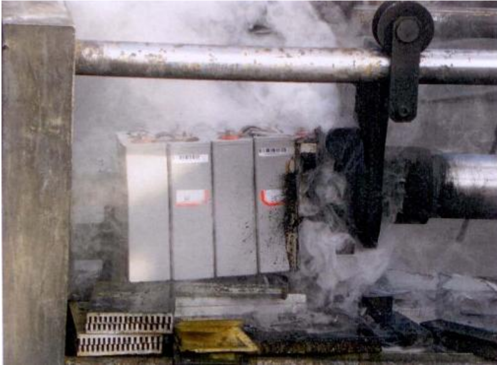
C12 Battery module's extrusion test
