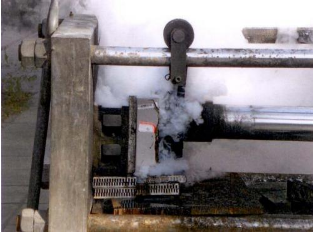
C1 Cell's extrusion test
