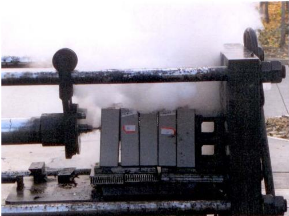
C13 Battery module's nail puncture test
