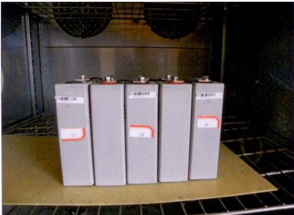
C11 Battery module's heating test
