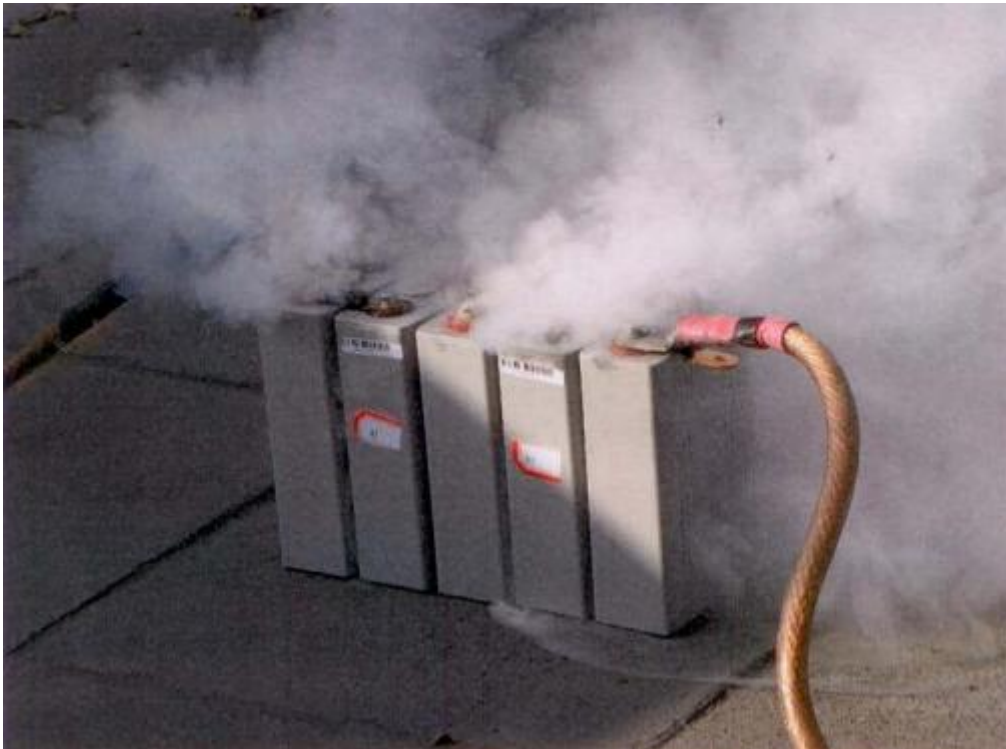
C10 Battery module's short-circuit test
